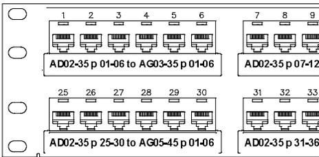
This can be interpreted as the near end set of six port as being located in a patch panel 35 rack units from the bottom of rack or cabinet at grid location AD02 and these ports are going to the "far-end" set of six ports located in a patch panel 35 rack units from the bottom of rack or cabinet at grid location AG03.
