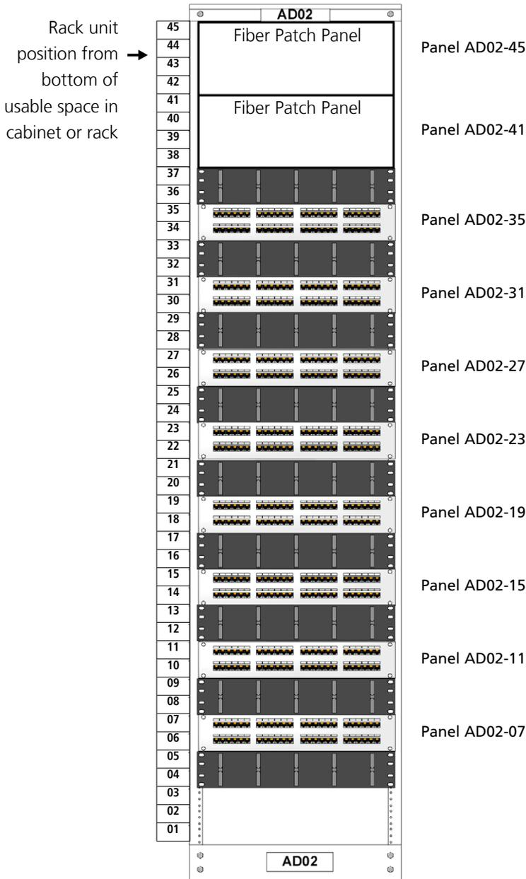
NOTE: The standard also allows the marking of panels and sub-panels using alpha characters starting with A and excluding "I", "O" and "Q" as outlined in sections 5.1.3.1.1 and 5.1.4.1.
