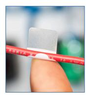
**3.** Wrap label and clear tail around wire to laminate the printed portion.
