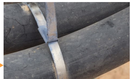
▶ Image shows blue coating fading from stainless steel cable tie.
